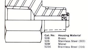
316 S.S. HEX COMPILES TO THE FOLLOWING SPECIFICATIONS ASTM-A276, ASTM-A182 OR QQ-S-763 MONEL HEX. COMPLIES TO QQ-N-281 (FEDERAL) **SPECIFICATION**
